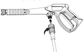
Connect the high pressure hose to the pump
