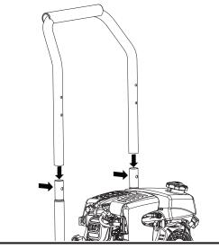
Install the storage panel and trigger handle
