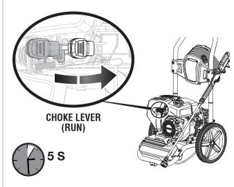
Move the choke lever fully to the right to Stop, then turn the fuel valve Off. (see page 11)
