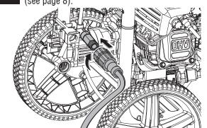
Completely uncoil and straighten high pressure hose to prevent kinks.
